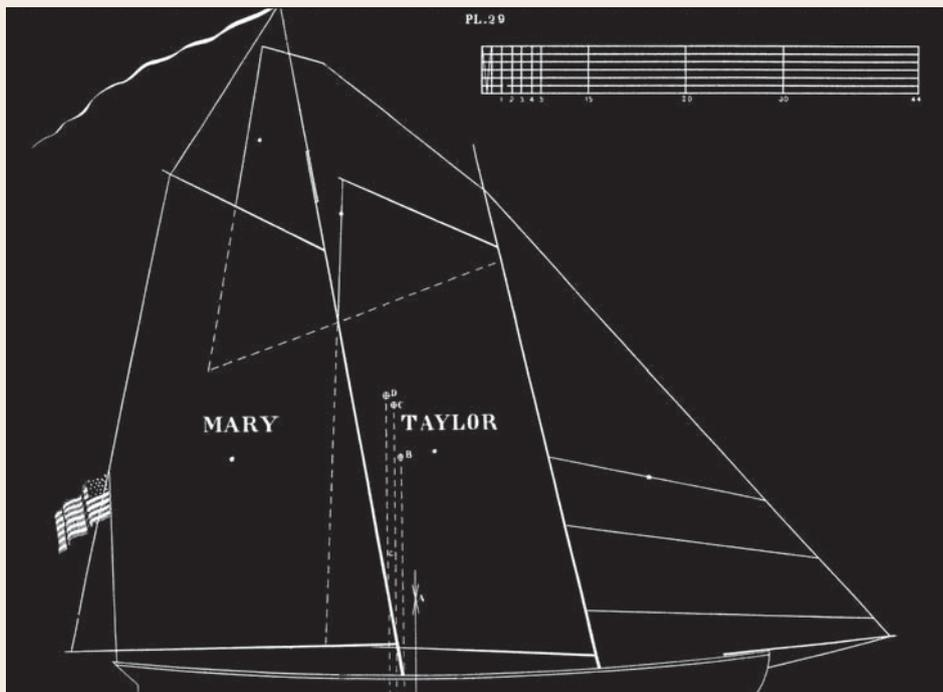
**Fig. 10:** Sail plan of New York pilot schooner, *Mary Taylor*, designed and built by George Steers in 1849. Plate 29 in John W. Griffith's *Treatise on Marine and Naval Architecture*, 3rd ed. (New York: Appleton & Co. 1852). The three lower sails are virtually identical to *America's* sails in figure 2.
